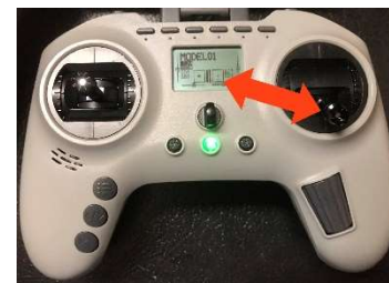
Figure 7. Channel Monitor Shows Right Gimbal Linked to Thrust
